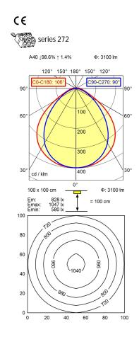
light source LED work equipment without 230V, 50/60Hz connected load env. 40 W power consumption luminous flux approx. 3.100 lm luminous efficiency approx. 78 lm/W light distribution direct direct ratio approx. 99 % 100° beam angle colour temperature neutral white colour temperatur approx. 5.000 K color rendering index (CRI) >= 80 chromaticity tolerance LED < 4 SDCM
