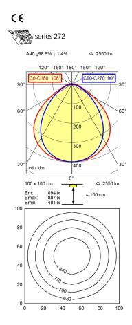
light source LED work equipment without 230V, 50/60Hz connected load env. 32 W power consumption luminous flux approx. 2.550 lm luminous efficiency approx. 80 lm/W light type/-color cold white approx. 5.000 K colour temperatur CRI > 80 color rendering index light distribution direct direct ratio approx. 99 % 100° beam angle chromaticity tolerance LED < 4 SDCM glare control diffuser foil luminance (L65)  $<= 17000 \text{ cd/m}^2$ unified glare rating (4H 8H) <= 25 system of protection IP 67
