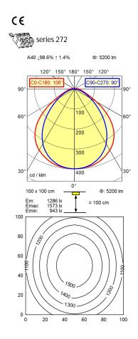
light source LED work equipment without 230V, 50/60Hz connected load env. 64 W power consumption luminous flux approx. 5.200 lm luminous efficiency approx. 81 lm/W light distribution direct direct ratio approx. 99 % 100° beam angle colour temperature neutral white colour temperatur approx. 5.000 K color rendering index (CRI) >= 80 chromaticity tolerance LED < 4 SDCM glare control diffuser foil luminance (L65)  $<= 18000 \text{ cd/m}^2$ unified glare rating (4H 8H) <= 25
