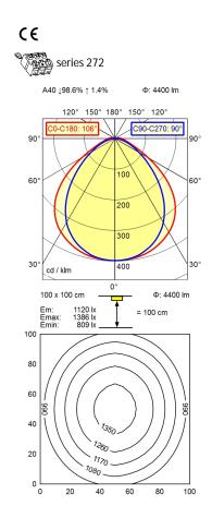
light source LED work equipment without 230V, 50/60Hz connected load env. 56 W power consumption luminous flux approx. 4.400 lm luminous efficiency approx. 79 lm/W light distribution direct direct ratio approx. 99 % 100° beam angle colour temperature neutral white colour temperatur approx. 5.000 K color rendering index (CRI) >= 80 chromaticity tolerance LED < 4 SDCM glare control diffuser foil luminance (L65)  $<= 17000 \text{ cd/m}^2$
