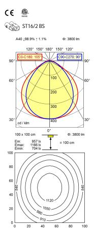
light source LED work equipment without connected load 22-26 V, DC env. 50 W power consumption luminous flux approx. 3.800 lm luminous efficiency approx. 76 lm/W light distribution direct direct ratio approx. 99 % 100° beam angle colour temperature neutral white colour temperatur approx. 5.000 K
