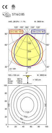
light sourceLEDwork equipmentwithoutconnected load22-26 V, DCpower consumptionenv. 50 Wluminous fluxapprox. 3.800 lmluminous efficiencyapprox. 76 lm/Wlight distributiondirect
