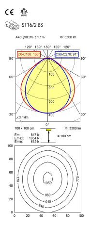
light source LED work equipment without connected load 22-26 V, DC env. 44 W power consumption luminous flux approx. 3.300 lm luminous efficiency approx. 75 lm/W light distribution direct direct ratio approx. 99 % 100° beam angle colour temperature neutral white colour temperatur approx. 5.000 K
