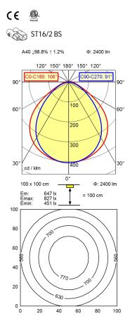
light source LED work equipment without connected load 22-26 V, DC env. 31.5 W power consumption luminous flux approx. 2.400 lm luminous efficiency approx. 75 lm/W light distribution direct direct ratio approx. 99 % 100° beam angle
