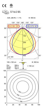
light source LED work equipment without connected load 22-26 V, DC env. 12.5 W power consumption luminous flux approx. 950 lm luminous efficiency approx. 73 lm/W light distribution direct direct ratio approx. 99 %
