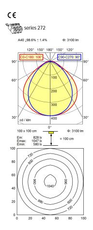
light source LED work equipment without 230V, 50/60Hz connected load env. 40 W power consumption luminous flux approx. 3.100 lm luminous efficiency approx. 78 lm/W light distribution direct direct ratio approx. 99 % 100° beam angle colour temperature neutral white colour temperatur approx. 5.000 K color rendering index (CRI) >= 80 chromaticity tolerance LED < 4 SDCM glare control diffuser foil luminance (L65)  $<= 17000 \text{ cd/m}^2$ unified glare rating (4H 8H) <= 25
