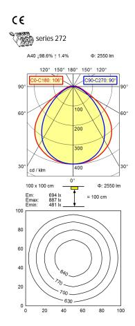
light source LED work equipment without connected load 230V, 50/60Hz env. 32 W power consumption luminous flux approx. 2.550 lm luminous efficiency approx. 80 lm/W light type/-color cold white colour temperatur approx. 5.000 K CRI > 80 color rendering index light distribution direct direct ratio approx. 99 % 100° beam angle chromaticity tolerance LED < 4 SDCM glare control diffuser foil luminance (L65)  $<= 17000 \text{ cd/m}^2$ unified glare rating (4H 8H) <= 25
