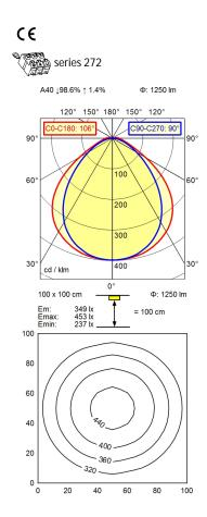
light source LED work equipment without 230V, 50/60Hz connected load env. 16 W power consumption luminous flux approx. 1.250 lm luminous efficiency approx. 78 lm/W light distribution direct direct ratio approx. 99 % 100° beam angle colour temperature neutral white colour temperatur approx. 5.000 K color rendering index (CRI) >= 80 chromaticity tolerance LED < 4 SDCM glare control diffuser foil luminance (L65)  $<= 16000 \text{ cd/m}^2$ unified glare rating (4H 8H) <= 25
